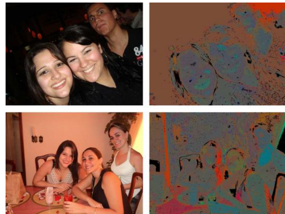
Fig. 2. Example illuminant maps for an original image (top) and a spliced image (bottom). The illuminant maps are created with the IIC-based illuminant estimator.
